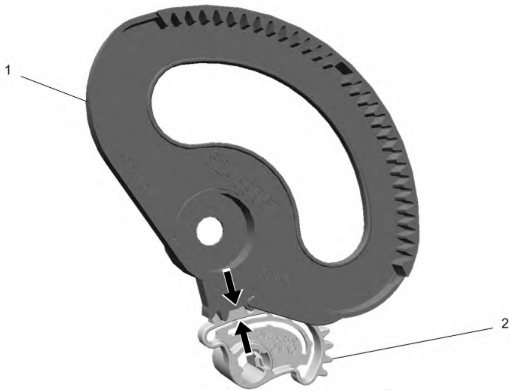
Fig. 197: Temperature Valve Gear And Mode Valve Lever Courtesy of GENERAL MOTORS COMPANY
